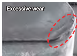
Existing grade (K10)
