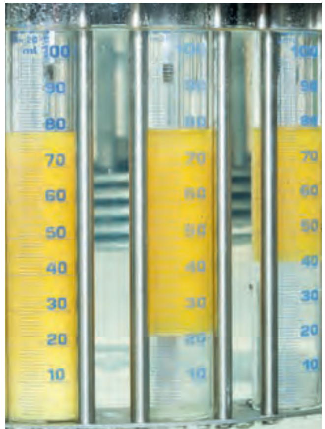
The laboratory test shows the water separation capability of various lubricating oils after five minutes. To the left is the non-optimized, commercially available circulating oil with process water. In the middle is standard oil with process water and to the right is the BECHEM Ovitool KT 460 S optimized for the process water with an outstanding water separation value.
