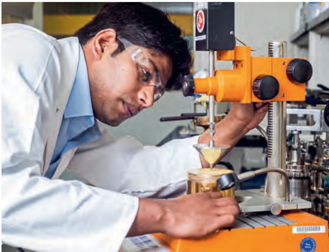
Testing at the CARL BECHEM Lubricants India lab: Worked penetration indicates the consistency of lubrication greases.
